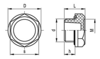
D = 44 d = G1 h = 13 L = 23 M = 31.0 s = 38 Tightening (N m) = 12-15
